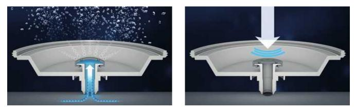
Oscillating non return valve ensures that the non return valve is not blocked with any dirt.
