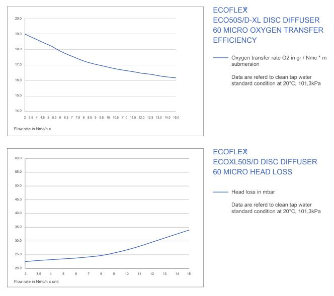
Comparable values can only be obtained with a similar setup and condition. Depending on the tank geometry, slit chart, water depth and planar allocation, the quoted values can change. All data are based on clean water 20°C temperature, 1013mbar / 68°F, 101,3kpa All data are approximate data!
